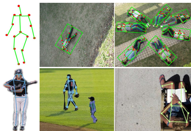
FIGURE 3. Fifteen-joint skeleton obtained after manually outlying each human body in our dataset (in the first row), and seventeen types of keypoints in MS COCO (person, in the second row), similarly.
