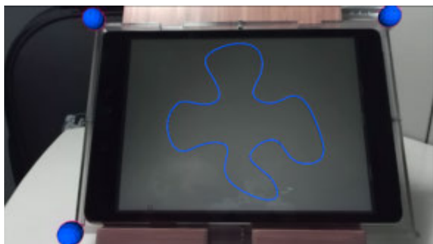
(b) Augmented reality of the tablet with the virtual spline registered onto the surface of the tablet display.
