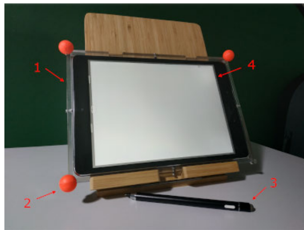
FIGURE 3. The tablet PC used in the user study. 1→Rigid shell for the tablet PC. 2→Fluorescent markers for the optical tracking. 3→Digital pen. 4→Tablet PC.
