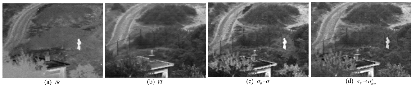
FIGURE 10. (a) and (b) are the IR and VI image respectively, (c) and (d) are the fusion results obtained by setting \sigma_B = \sigma and \sigma_B = 4\sigma_{gau}^L , respectively.
