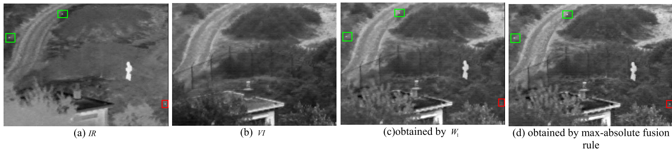
FIGURE 8. (a) and (b) are the IR and VI image respectively, (c) and (d) are the fusion results obtained by using the weights W_1 and the max-absolute fusion rule, respectively.
