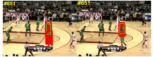
FIGURE 6. Comparison before and after the addition of the deviation screening strategy. The red and green boxes are the sample candidate box and ground truth, respectively. Before the screening strategy is added, the sample candidate box is distributed around the target and the mendacious similar targets. After the screening strategy is added, the sample candidate box is only distributed around the target.
