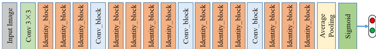
FIGURE 3. The detailed architecture of classification network.
