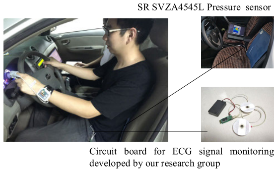
FIGURE 2. Experimental setup for the measurement of heartbeat signal during driving.
