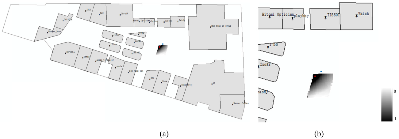
FIGURE 15. Positioning result for Implicitly-Scene3-1 in F1: “front 15 m is TISSOT, left 15 m is ZuokY, left-front is I DO. The participant is approximately 16.5 m away from TISSOT. (a) Global, (b) Local.
