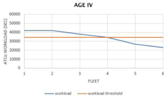
FIGURE 7. Results from Case Study IV: variation in ATCo workload (in seconds) considering different fleets at TML age IV.
