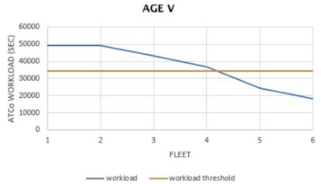
FIGURE 8. Results from Case Study V: variation in ATCo workload (in seconds) considering different fleets at TML age V.
