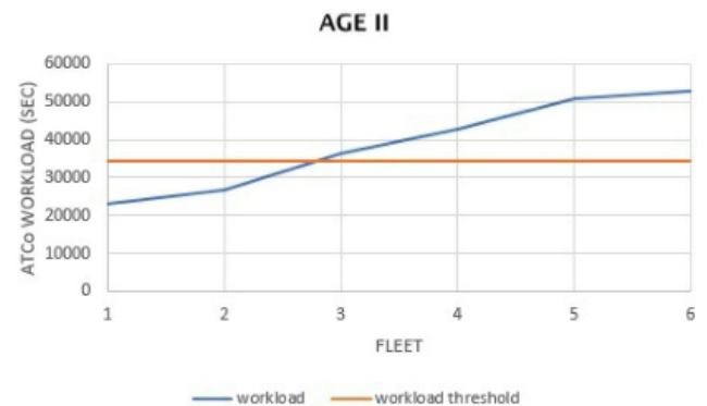
FIGURE 5. Results from Case Study II: variation in ATCo workload (in seconds) considering different fleets at TML age II.
