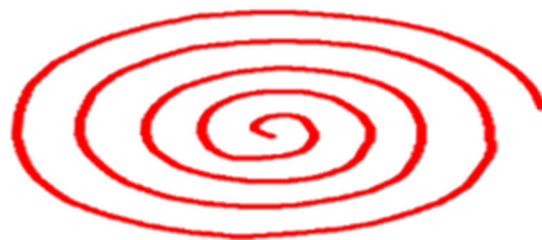
FIGURE 6. Design of pan-cake channel flow pattern.
