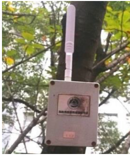
( a ) the sensor node of JNSN
