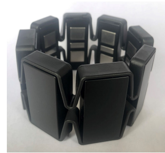
FIGURE 4. The armband sensor named MYO was adopted to measure the related major EMG signal.
