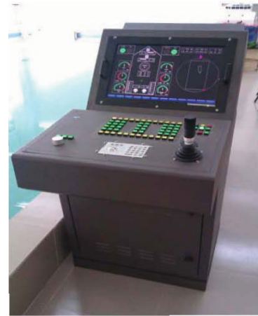
FIGURE 5. Practicality picture of ship control system.
