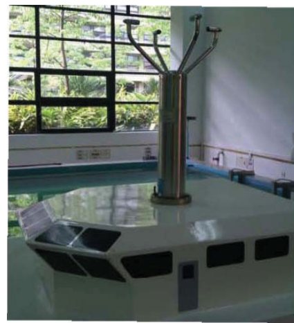
FIGURE 6. Mounting image of attitude sensor and mounting image of wind sensor.
