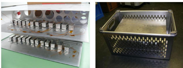
(a) DUTs mounted onto the trays for irradiation. (b) Ventilated box with DUT trays.
