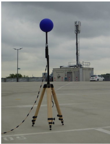
FIGURE 2. Measurement site in in LOS of a 5G NR base station situated on the upper level of a parking building in Düsseldorf, Germany.
