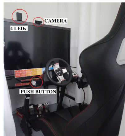
FIGURE 3. Driving simulator with LED reaction time task setup and camera for video recording.
