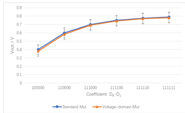
FIGURE 8. Comparisons of Voltage-domain Approximate Multiplication and Standard Multiplication (With Fixed Input).
