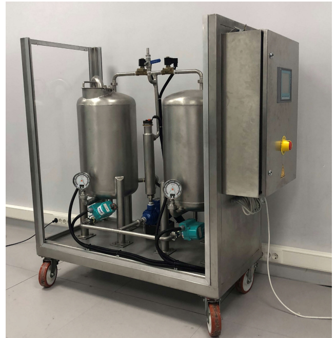
FIGURE 3. Water level control automation components.
