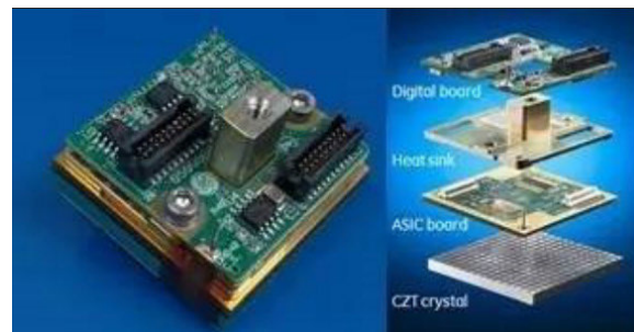
FIGURE 5. The new CZT detector.
