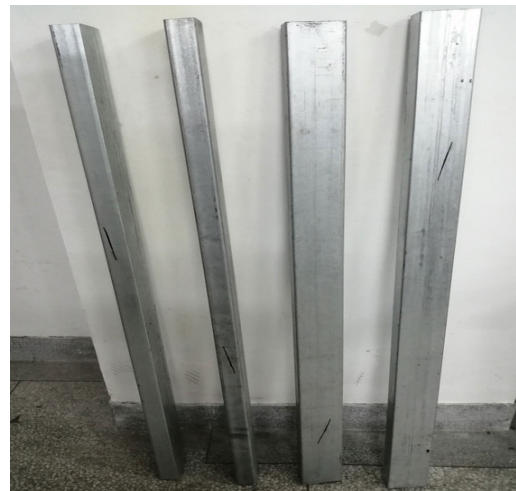
FIGURE 15. Girder specimens with crack.
