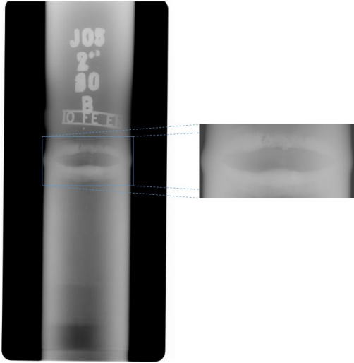
FIGURE 14. Image of the pipe, highlighting the weld bead clipping.
