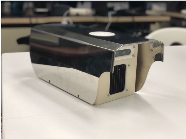
FIGURE 1. Prototype of the marine data collection device. Data such as visible light, infrared radiation (IR), inertial measurement unit (IMU), and GPS are saved simultaneously.
