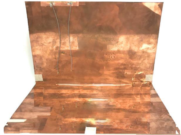
FIGURE 6. Photo of the fabricated 5G four-element MIMO antenna system integrated with the laptop.
