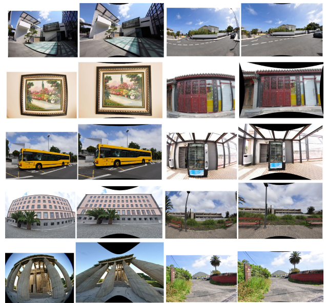
FIGURE 8. Correction of some challenging real images from previous papers on distortion estimation [33], [34]. Column 1 and column 3 are original distorted images. Column 2 and column 4 are corresponding undistorted images using parameters estimated by our proposed method.
