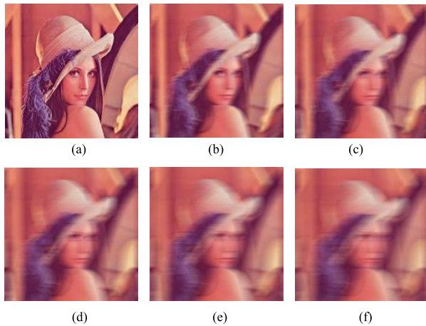
FIGURE 8. Blurred images obtained by moving Lena with different distance. (a) Original image; (b) Len =11; (c) Len = 15; (d) Len = 19; (e) Len =21; (f) Len = 27.
