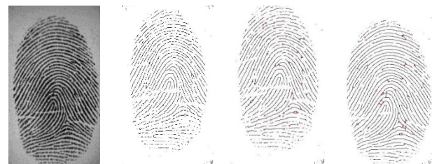
(A) initial image (B) skeletonization (C) minutiae of template (D) minutiae of sample
