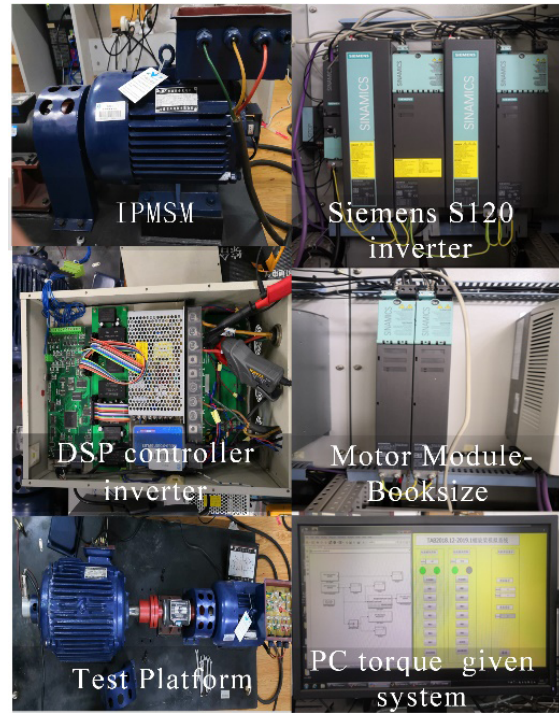
FIGURE 9. Schematic diagram of the experimental platform.
