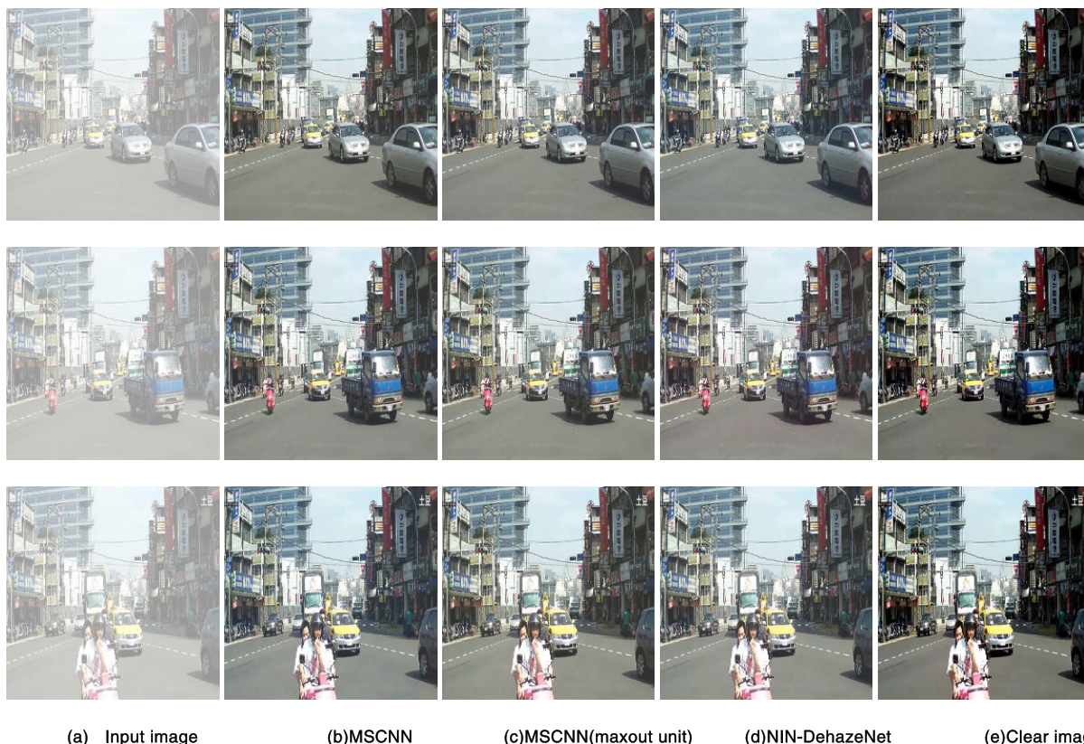
FIGURE 4. Three images were selected from 100 images, and we obtained a fog-free image with MSCNN, improved MSCNN which extracting features by maxout unit and NIN-DehazeNet.
