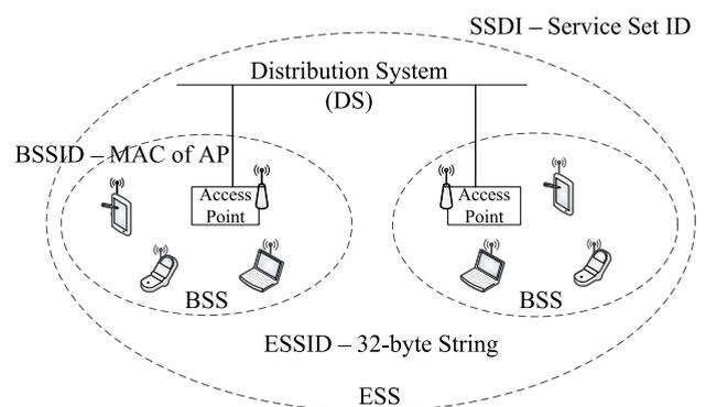
FIGURE 2. Extended service set architecture.
