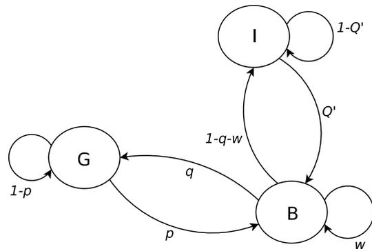
FIGURE 12. Three state packet loss model [144].
