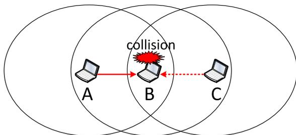
FIGURE 7. Collision scenario of Wi-Fi networks.
