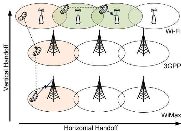
**FIGURE 5. Vertical and horizontal handoffs.**
