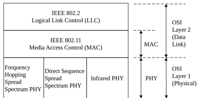
FIGURE 1. Standard for MAC and physical layer for WLANs.
