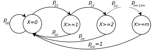
FIGURE 14. Loss run-length model with unlimited state space ( $m \rightarrow \infty$ ) [146].
