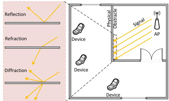
**FIGURE 6. Signal propagation in wireless environments: reflection, refraction and diffraction.**
