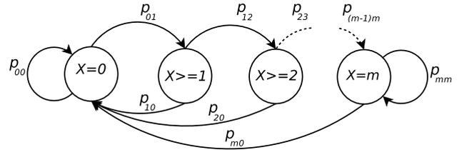
FIGURE 15. Loss run-length model with limited state space [146].
