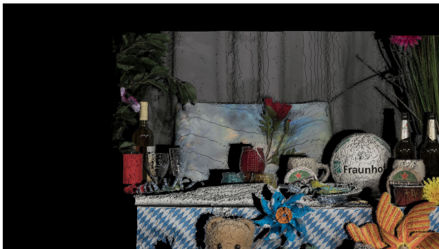
FIGURE 7. Warping a reference view to a faraway camera position produces only a partial reconstruction. Similar to Figure 6 black regions correspond to pixels which are not seen by the camera at the reference view location. The above image is the result of warping the reference view X(20, 98) to the camera position of the target view X(4, 2) . Since the reference view resides on the lower right corner of the camera array, the upper and left parts of the view at the target location cannot be reconstructed using warping of the reference view alone.
