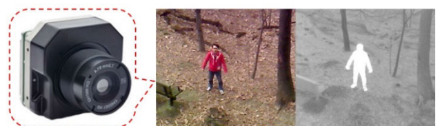
FIGURE 1. Example of a thermal camera, a visible light image, and a thermal image, respectively, from left to right.
