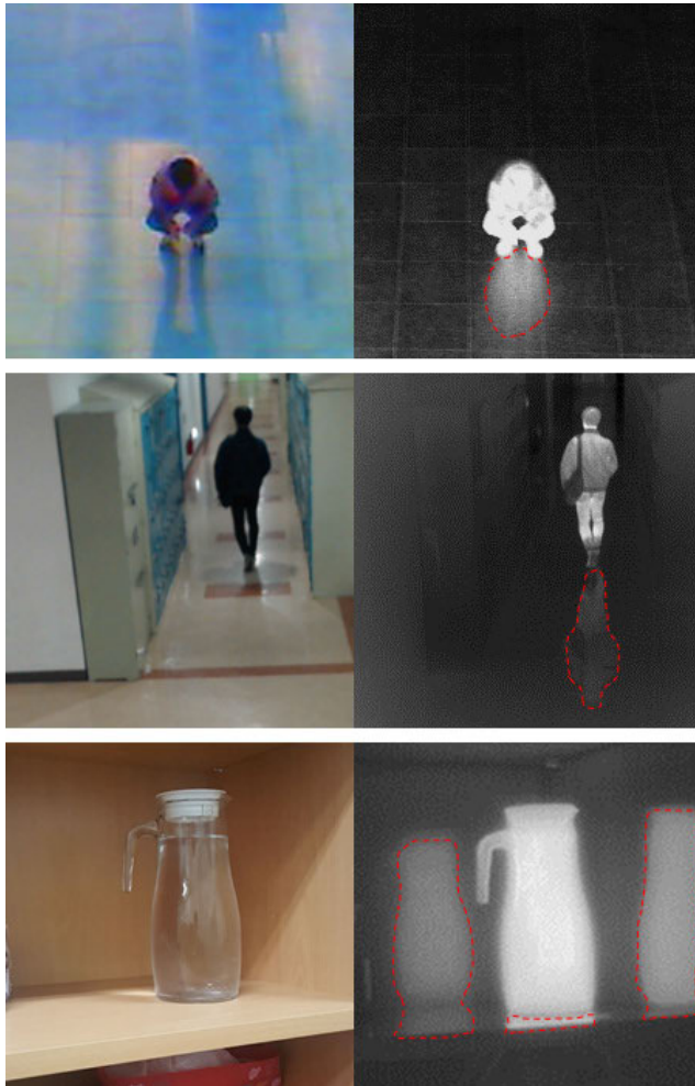
FIGURE 2. Examples of thermal reflections. Left and right figures show visible light images and the corresponding thermal images.
