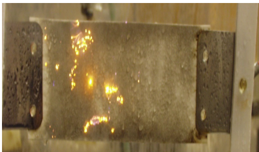
FIGURE 4. Specimen surface state during the salt-fog test.
