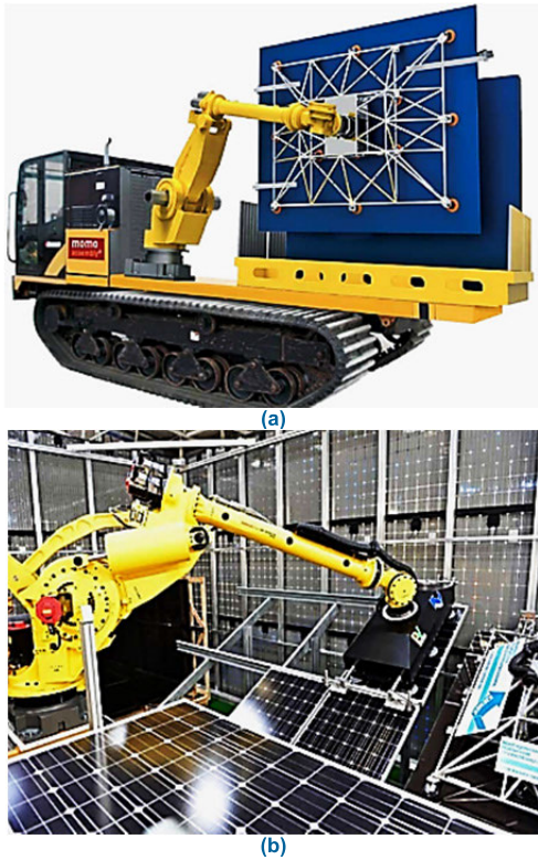
FIGURE 10. MOMO Robotic System – Handling of PV modules [120]: (a) Transportation (b) Assembly.
