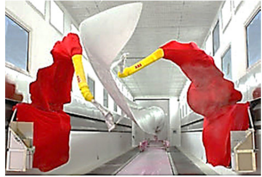
FIGURE 17. Robots painting wind turbines [165].
