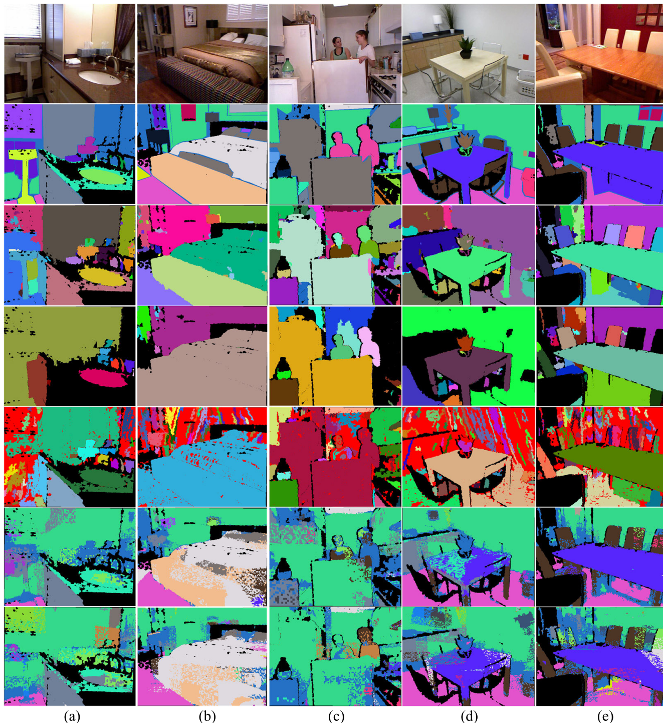
FIGURE 16. Comparison of segmentation result on point clouds from NYU-v2 database. From top to bottom: scene images, groundtruth, results from ours, LCCP, RG, PointNet++ and RSNet. LCCP under-segments the point cloud, RG over-segments the each object to several parts with miscellaneous points. The deep learning based methods PointNet++ and RSNet generate ambiguous segmentation labels and unspecific segmenting boundaries. Ours achieves the best segmentation and separates each object correctly, comparing to the groundtruth. Parameters: R_{voxel} = 0.01 , R_{patch} = 0.08 , \beta_{th} = 10^\circ .
