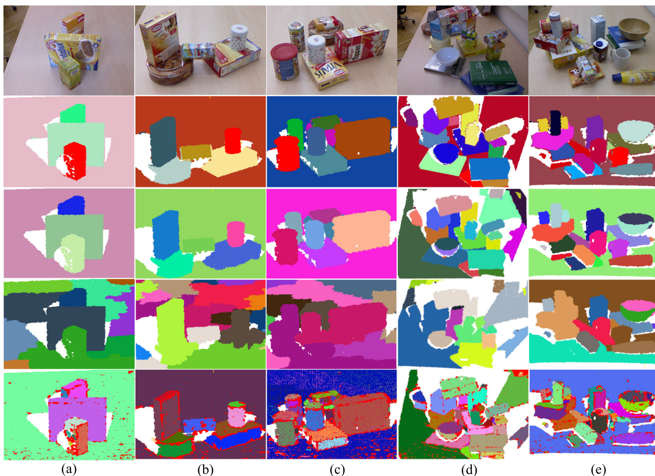
FIGURE 15. Comparison of segmentation result on point clouds from OSD-v0.2 database. From top to bottom: scene images, groundtruth, results from ours, LCCP, and RG. RG over-segments the each object to several parts with miscellaneous points. LCCP under-segments the point cloud, especially for simple scenes. Ours achieves the best segmentation and separates each object correctly, comparing to the groundtruth. Parameters: R_{voxel} = 0.007 , R_{patch} = 0.06 , \beta_{th} = 10^\circ .
