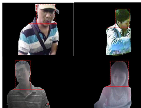
FIGURE 6. Head location results (indicated in red boxes) in sideview condition in a real ATM scene.
