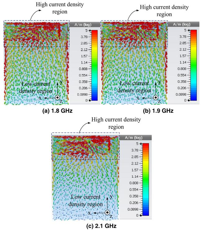
FIGURE 4. Current distribution of the far-field segment of the antenna.
