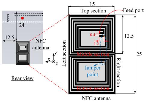
FIGURE 5. Configuration of dual-loop NFC antenna on the rear of the FF antenna (unit: mm).
