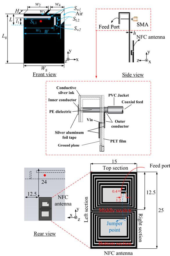
FIGURE 10. Configuration of the proposed FNFC antenna (not to scale).
