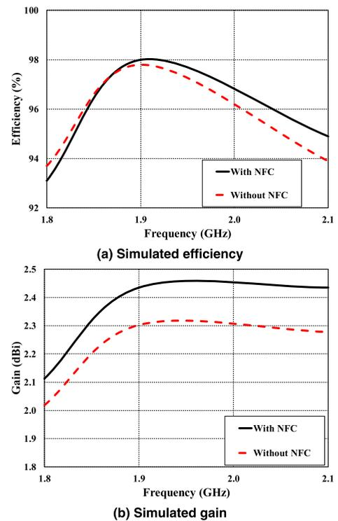
FIGURE 8. Comparison between the FF antenna with and without dual-loop NFC.
