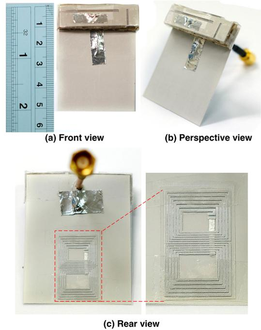
FIGURE 11. The prototype of integrated FNFC antenna.
