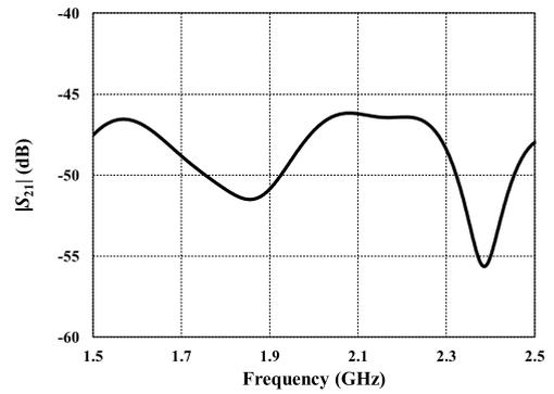
FIGURE 7. Simulated isolation  $|S_{21}|$  of the integrated FNFC antenna.
