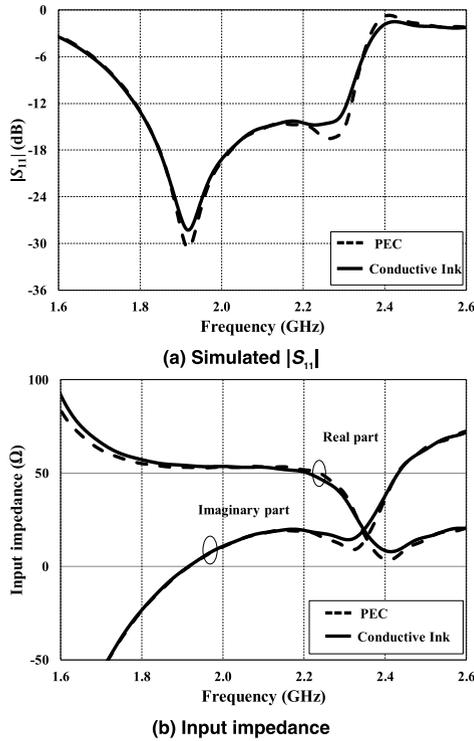
FIGURE 2. Comparison between conductive silver ink and PEC of the far-field segment.
