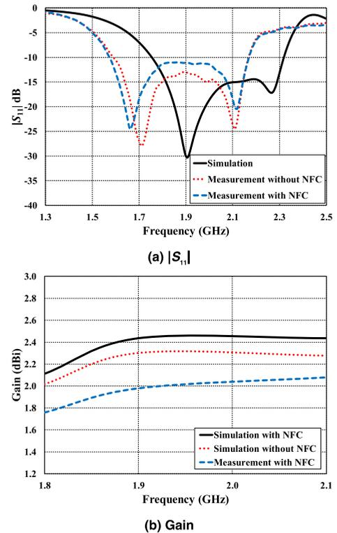
FIGURE 12. Simulated and measured  $|S_{11}|$  and gains of the integrated FNFC antenna.
