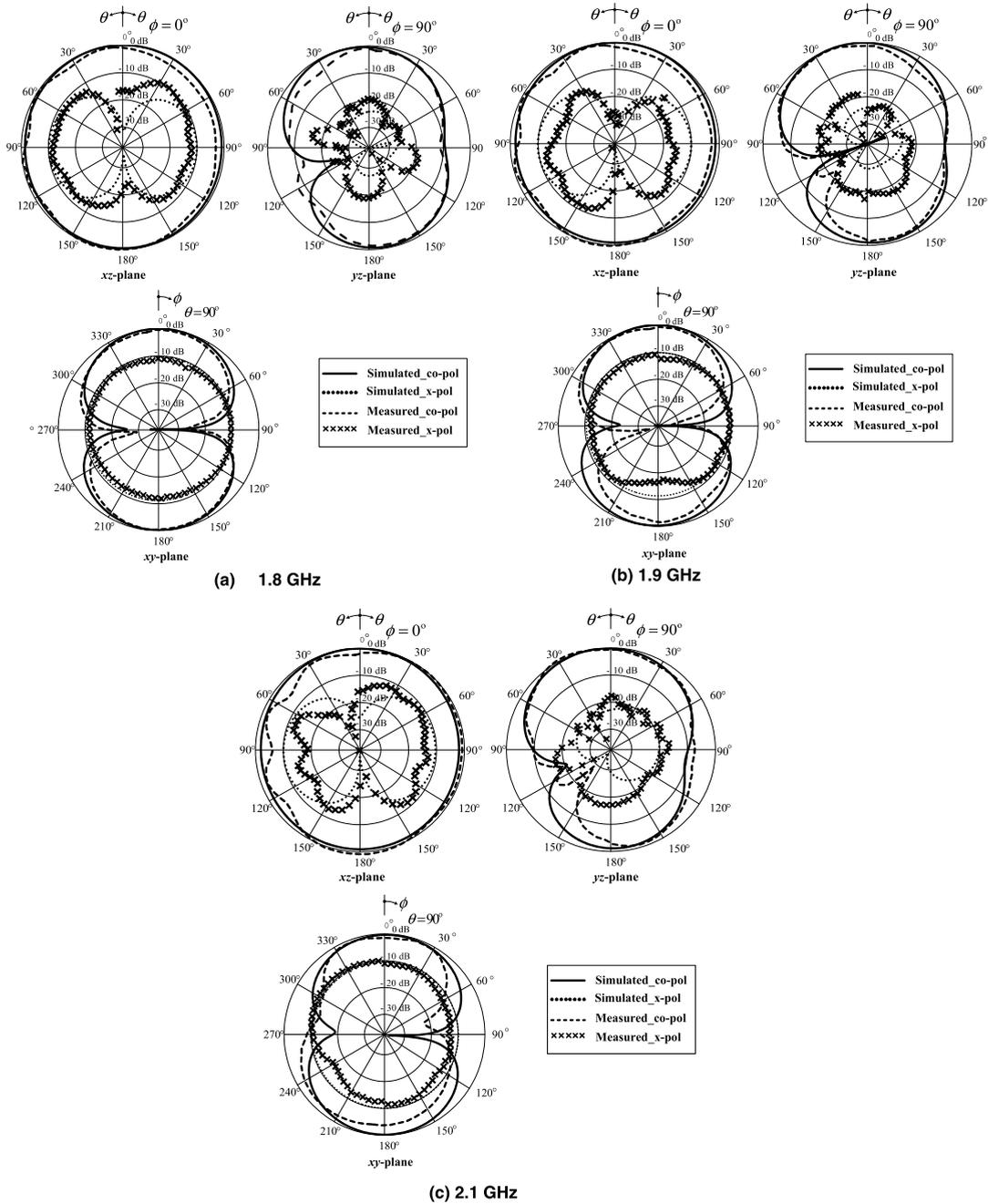
**FIGURE 13.** Simulated and measured radiation patterns of the integrated FNFC antenna (simultaneously operated between NFC and FF antennas).
