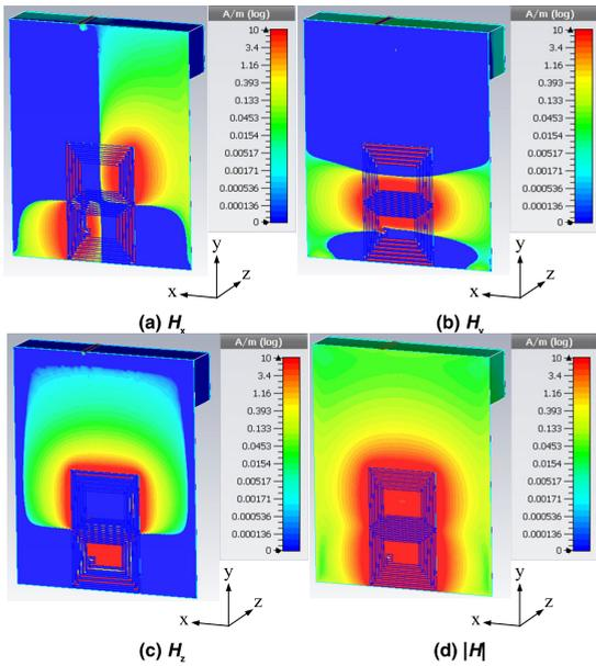
FIGURE 9. Magnetic field distribution of dual-loop NFC given the frequency of 13.56 MHz (simultaneously operated between NFC and FF antennas).
