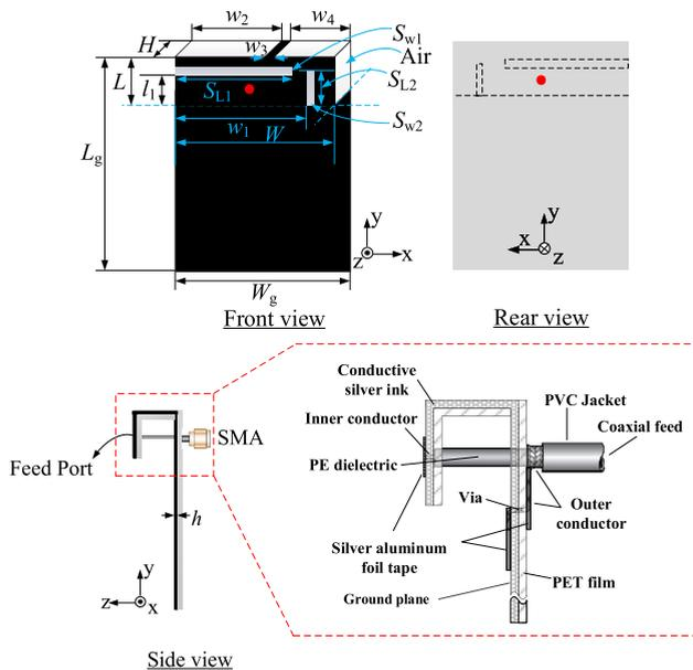
**FIGURE 1.** Configuration of the far-field segment of integrated FNFC antenna.
