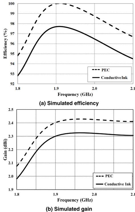
FIGURE 3. Comparison between conductive silver ink and PEC of the far-field segment.
