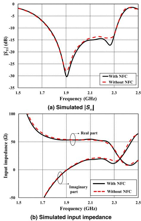
FIGURE 6. Comparison between the FF antenna with and without dual-loop NFC.
