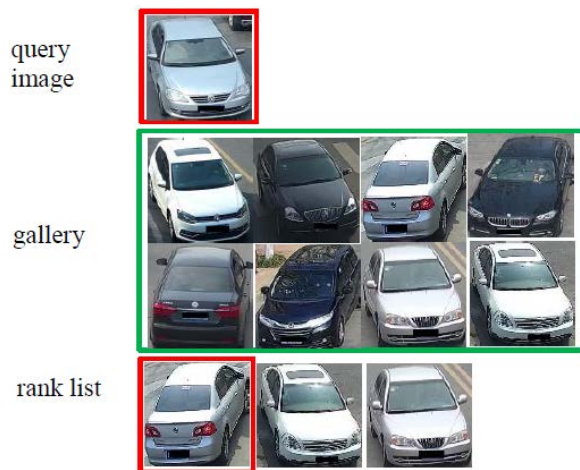
FIGURE 1. Explanation of vehicle re-identification task. The query image is compared with many vehicle images captured by multiple cameras (i.e. gallery), and get a rank list which contains matching vehicle images (images are selected from [92]).
