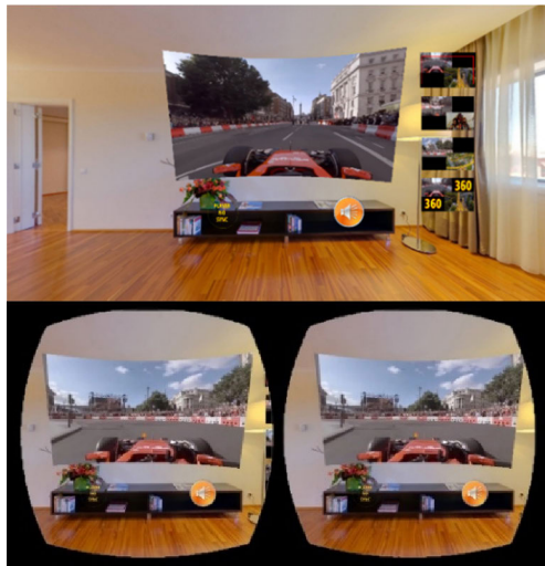
FIGURE 11. Immersive scenario seen through a flat display (top) and through a stereoscopic display or HMD (bottom).
