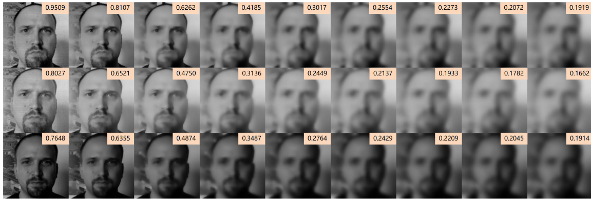
FIGURE 4. Scheme one iterative guided filter results on REPLAY-ATTACK databate, given in Eq.20. Average gradient (number in the boxes) showing the smooth degree of each iteration step of guided filter. From left to right, the image are filtered with different \varepsilon and fixed r, r = 4, \varepsilon^{(n)} = 0.05^2 \times 2^n . Samples cover three kind of face image in adverse illumination, from top to bottom: print attack, video attack and real face.
