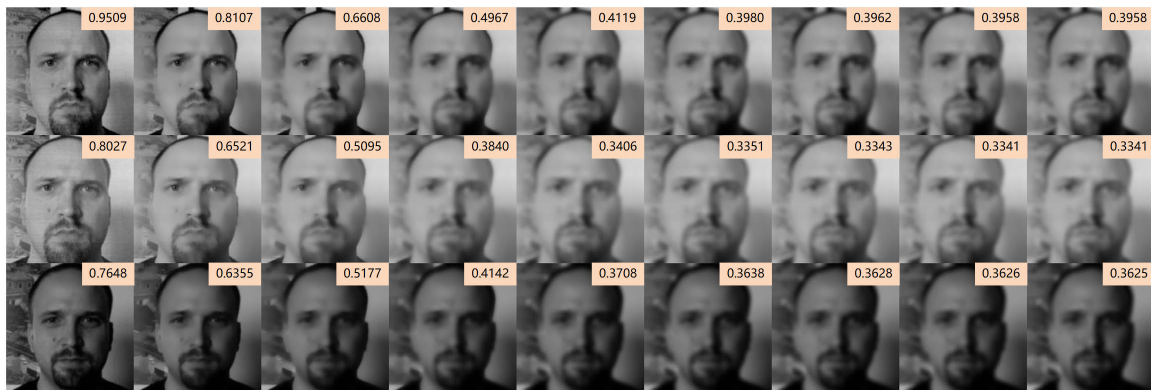
FIGURE 5. Scheme two iterative guided filter results on REPLAY-ATTACK databate, given in Eq.21. Average gradient (number in the boxes) showing the smooth degree of each iteration step of guided filter. From left to right, the image are filtered with different \varepsilon and fixed r, r = 4, \varepsilon^{(n)} = 0.05^2 \times 2^n . Samples cover three kind of face image in adverse illumination, from top to bottom: print attack, video attack and real face.
