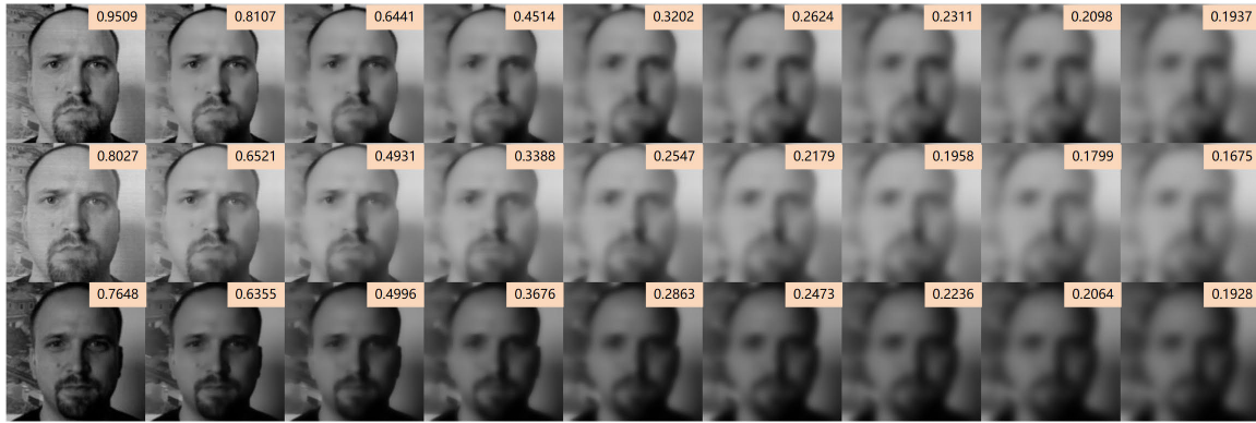
FIGURE 6. Scheme three iterative guided filter results on REPLAY-ATTACK databate, given in Eq.22. Average gradient (number in the boxes) showing the smooth degree of each iteration step of guided filter. From left to right, the image are filtered with different \epsilon and fixed r, r = 4, \epsilon^{(n)} = 0.05^2 \times 2^n . Samples cover three kind of face image in adverse illumination, from top to bottom: print attack, video attack and real face.
