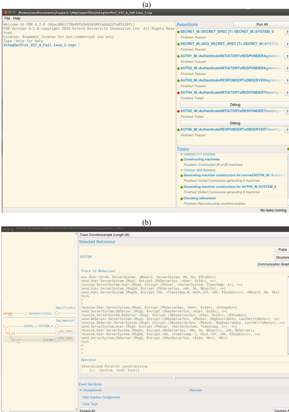
FIGURE 7. Checking failure protocol case 1 using FDR 4.2.0. (a) Failed authentication assertions; (b) Exploring the debug tree to the process SYSTEM.
