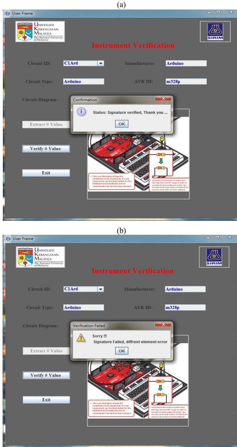
FIGURE 10. Screenshots of the prototype results. (a) ES's code is authentic; (b) ES's code is inauthentic.
