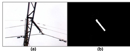
FIGURE 10. Insulator extraction. (a) original image. (b) insulator segmentation.
