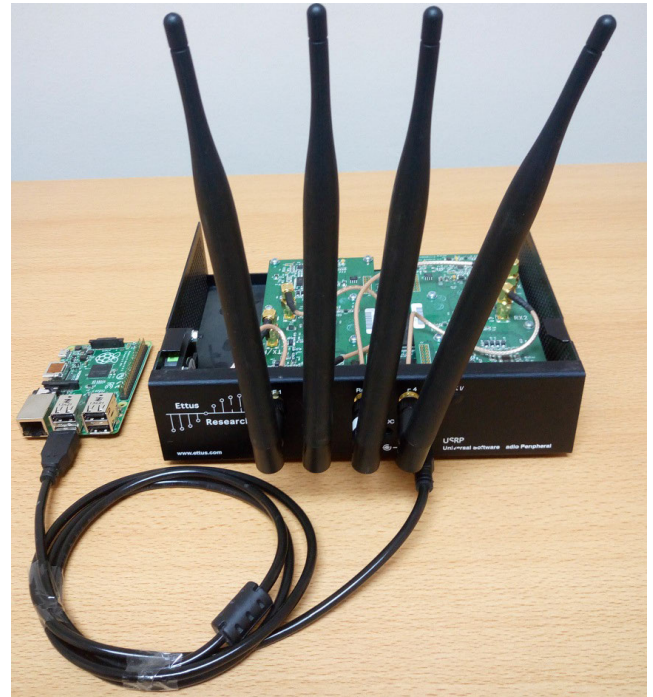
FIGURE 3. Example of a Raspberry Pi node connected to a USRP1 via a USB interface in WiPi.
