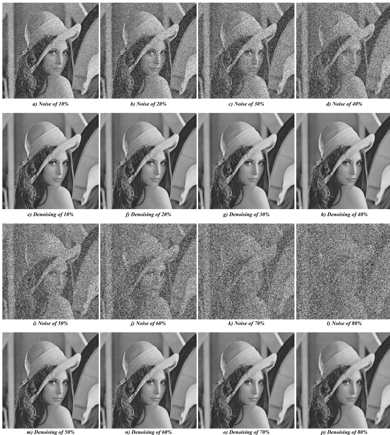
FIGURE 4. Denoising results by IMF for the Lena image with the size of 512 \times 512 pixels with different SPN ratios. a) (15.43 dB, 0.1758, 0.1362, 1, 0.9910), b) (12.42 dB, 0.0848, 0.0887, 1, 0.9789), c) (10.68 dB, 0.0533, 0.0673, 1, 0.9646), d) (9.42 dB, 0.0364, 0.0528, 1, 0.9494), e) (43.48 dB, 0.9913, 0.8974, 518.49, 1), f) (40.18 dB, 0.9796, 0.8106, 457.49, 0.9999), g) (37.05 dB, 0.9675, 0.7343, 425.55, 0.9999), h) (35.40 dB, 0.9541, 0.6653, 398.35, 0.9998), i) (8.44 dB, 0.0263, 0.0422, 1, 0.9333), j) (7.65 dB, 0.0182, 0.0325, 1, 0.9141), k) (6.99 dB, 0.0139, 0.0278, 1, 0.8979), l) (6.42 dB, 0.0092, 0.0213, 1, 0.8803), m) (33.98 dB, 0.9383, 0.5917, 357.47, 0.9997), n) (32.49 dB, 0.9183, 0.5135, 306.95, 0.9994), o) (31.23 dB, 0.8953, 0.4353, 266.22, 0.9990), p) (29.70 dB, 0.8623, 0.3445, 210.75, 0.9982).
