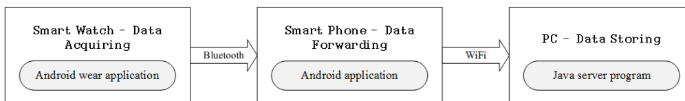
FIGURE 1. Structure of data acquisition system.
