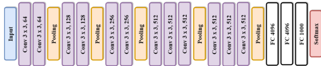
FIGURE 2. The basic architecture of VGGNet used in ILSVRC 2014 challenge. Different versions of VGGNet architecture have same basic structure, however the number of convolution layers changed in each architecture. Convolution layer is represented with ‘Conv’ and fully connected or dense layer with ‘FC’.
