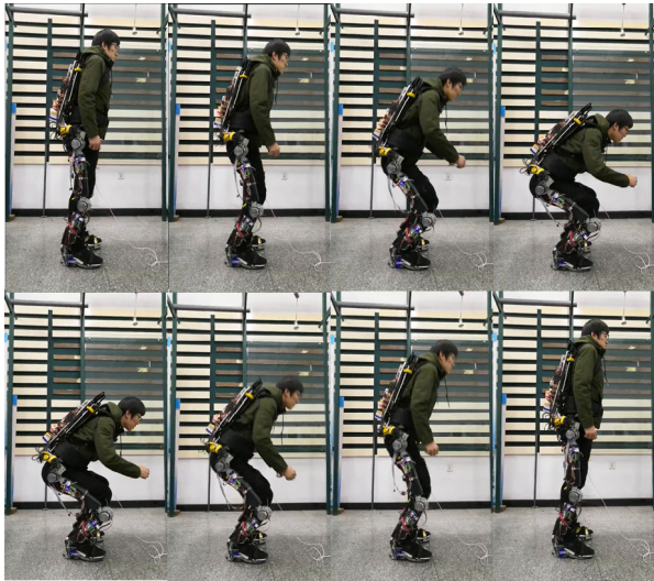
FIGURE 17. The experimental process of squatting down and standing up.
