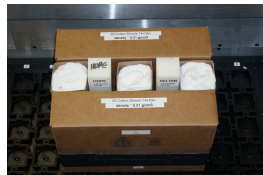
FIGURE 4. Experimental setup for measurements; a) top view showing the X-ray source, source collimator, and L-shaped array, three-target scenario (reconstructions in Fig. 8); markers show the origin of (x, y) coordinate system. A slit opening built into the detectors ensures that only in-plane scatter is measured; b) zoom on coaxial target (reconstructions in Fig. 9); c) zoom on box target (reconstructions in Fig. 11).
