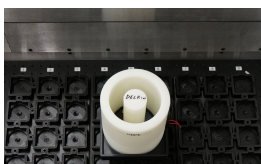
FIGURE 4. Experimental setup for measurements; a) top view showing the X-ray source, source collimator, and L-shaped array, three-target scenario (reconstructions in Fig. 8); markers show the origin of (x, y) coordinate system. A slit opening built into the detectors ensures that only in-plane scatter is measured; b) zoom on coaxial target (reconstructions in Fig. 9); c) zoom on box target (reconstructions in Fig. 11).
