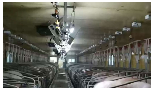
FIGURE 1. The installation of the depth camera to acquire the back of pigs in top-view images.
