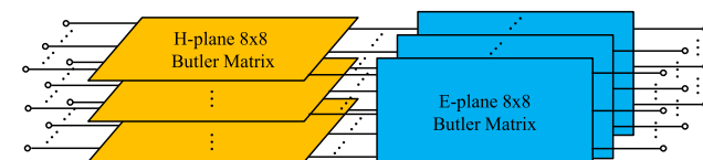
FIGURE 2. Conventional 64 × 64-way Butler matrix.
