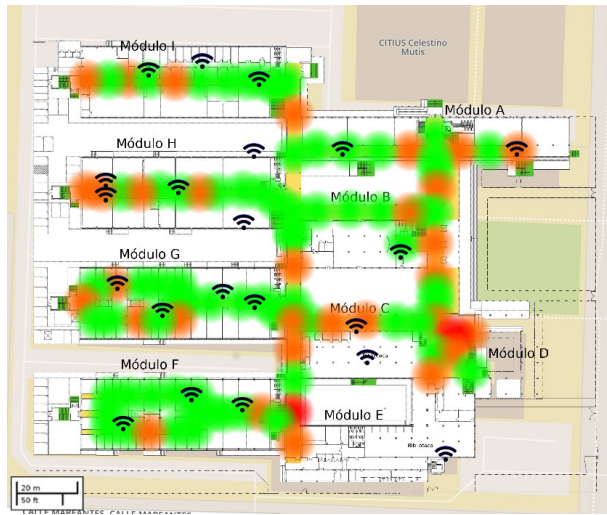
FIGURE 22. Localization results-heatmap floor 0 using regression KNN.
