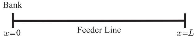
FIGURE 1. A single, straight-line distribution feeder that starts at a bank, through a finite-length line with length L , and ends at a non-loading terminal.
